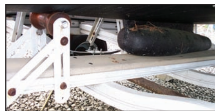
The new composite keel board for Paul's old boat trailer.
